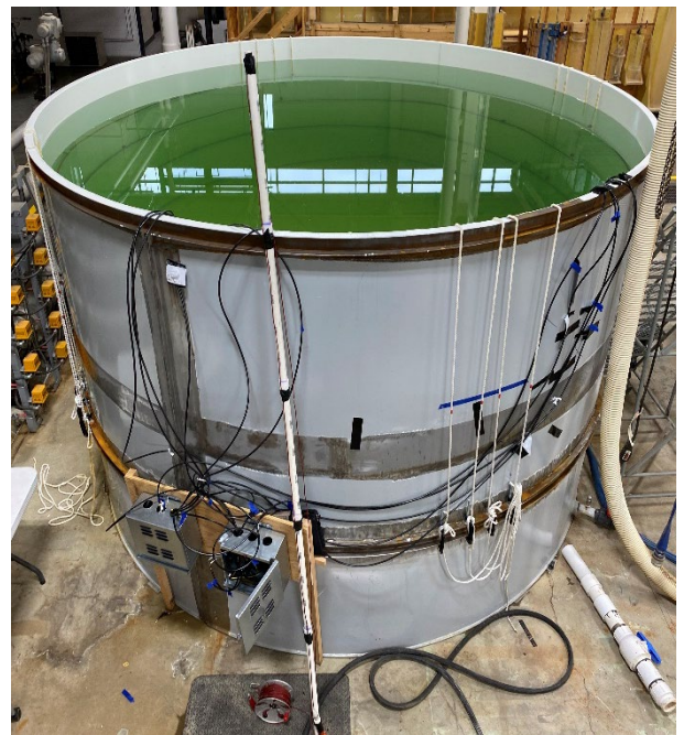
Laboratory scale model of a water storage tank with a cathodic protection corrosion mitigation system installed.
